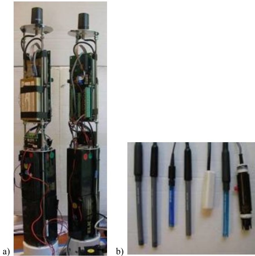
Figure 8. Continuous sensor units deployed for this study, including a) data loggers, cellular modems and batteries [casing removed], and b) individual probes for measuring pH, DO, temperature, electrical conductivity and turbidity.
